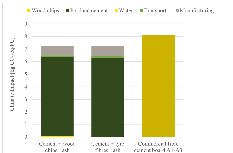
Fig. 11. Climate impact for the production stages (A1-A3) for the analysed composites compared with a commercial fibre cement board.
