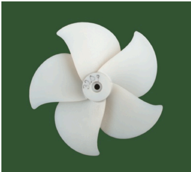
Fig. 6. The propeller geometry (pressure side).
