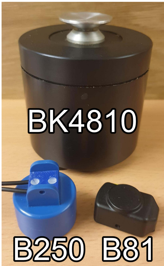
Figure 2 The transducers B250, Radioear B81 and the Minishaker (BK4810) showing their appearances and size differences. An adapter with the same shape as the B250 surface touching the skin is attached to the Minishaker.
