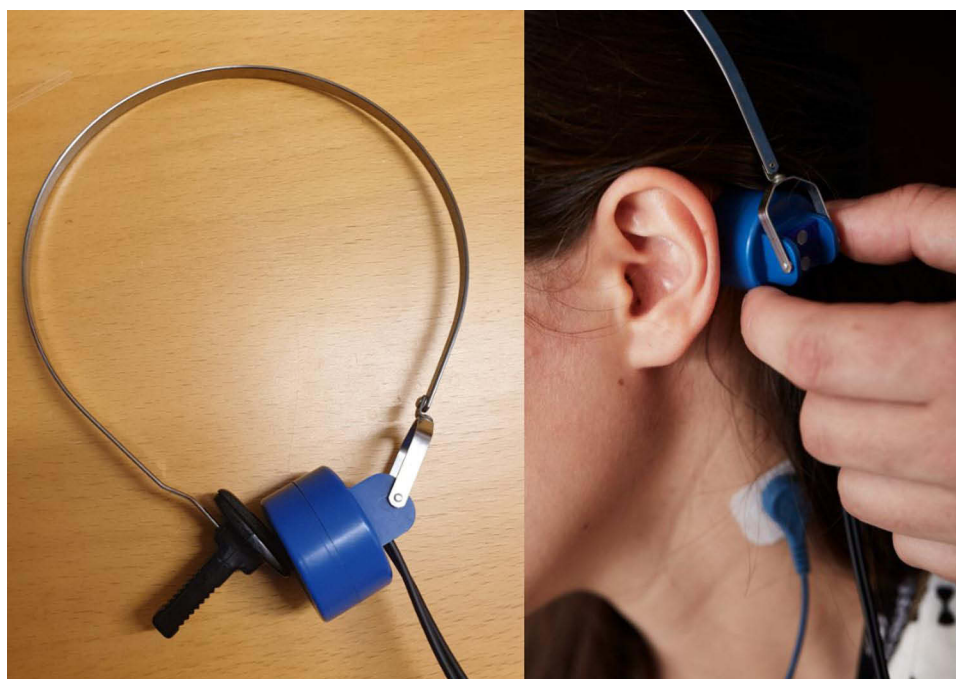
Figure 1 The B250 transducer appearance and how it is attached to the mastoid with a steel spring headband prior to cVEMP testing.
