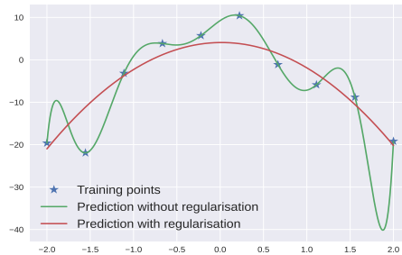
Figure 1.3: An illustration of overfitting with a model of the form Y_i = \sum_{k=0}^{10} \theta_k X_i^k + \xi_i where \xi_i is normal distributed noise with parameters \xi_i \sim N(0, 5^2) . Based on the 10 marked data points we see the prediction of both an OSL estimate (green line) and a lasso estimate with \lambda = 1 (red line).
