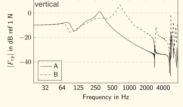
The increased TDR between 250 Hz and 2000 Hz indicates a lower sound radiation from the track.
