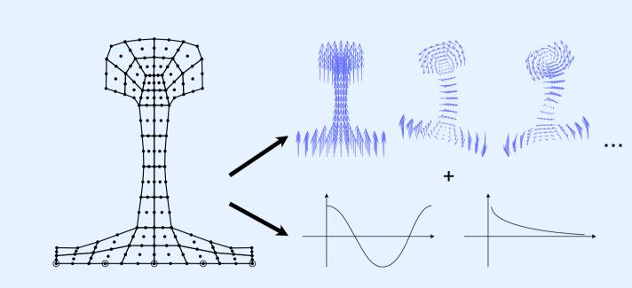
WFEM coupled to spring-mass-spring system at each rail seat  Receptance R under the rail foot is modeled as
