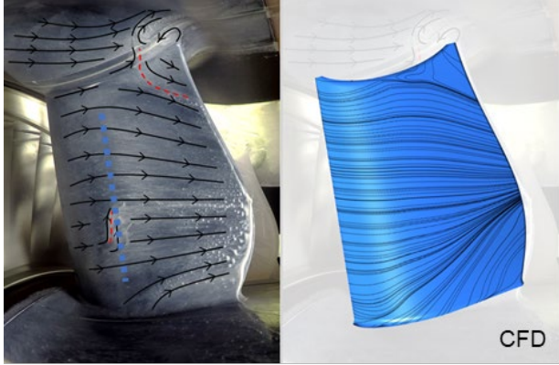
FIGURE 9: Oil-film visualization (left) and near-wall streamlines from CFD (right) on a bump OGV suction side at on-design flow coefficient ( FC=0.622 ).
