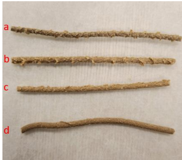
Figure 13. Extruded filaments of a) PP-TMP, b) PP-TMP AKD Hex, c) PP-TMP AKD Lau and d) PP-TMP AKD St.
