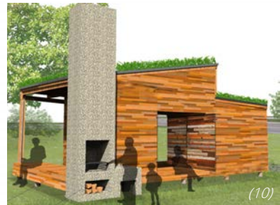
(Fig. 6:10) The BBQ chimney and pier foundation are made with 'tabby concrete.'
