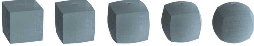
Fig. 4. Cube-sphere hybrid particles, in which the parameter \eta is, from left to right, 0.1, 0.3, 0.5, 0.7, and 0.9. The cube ( \eta = 0.0 ) and the sphere ( \eta = 1.0 ) are not shown.
