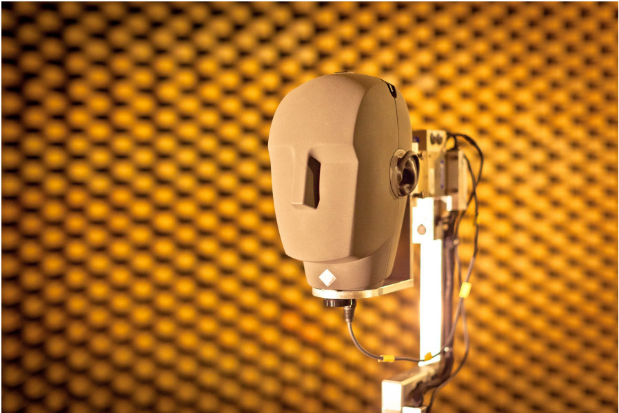
Figure 1.1: Neumann KU100 dummy head to capture HRIR data under free-field conditions in an anechoic chamber. Image from [4] licensed under CC BY 3.0.
