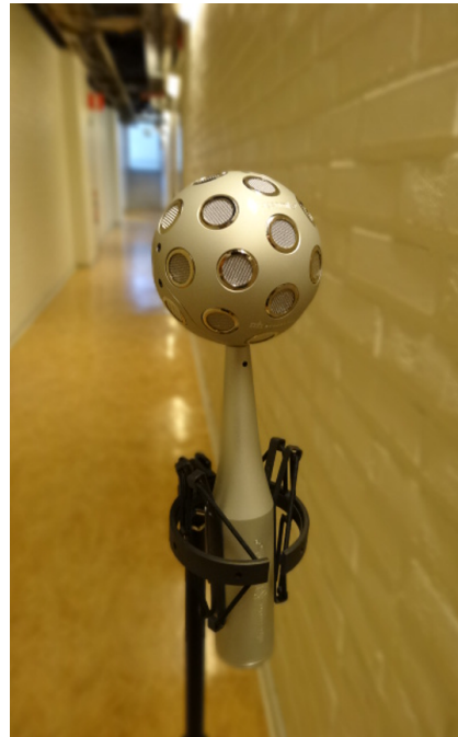
Figure 1.5: mh acoustics Eigenmike em32 SMA [16]. [Image: Jens Ahrens]
