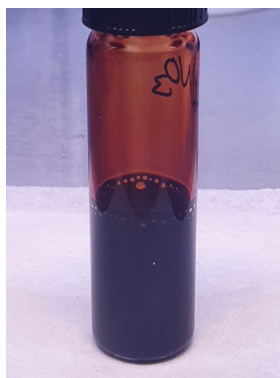
Figure 11 Image of catholyte, 5%wt \text{Li}_2\text{S}_8 in TEGDME with 0.4. M \text{LiNO}_3 .
