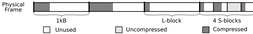
Figure 4.5: Main memory with a mixture of block types. Each 1kB space is one L-block or four s-blocks.
