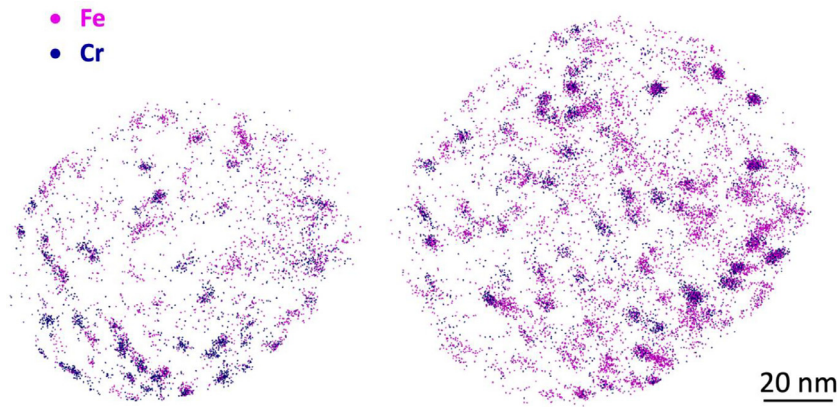
Fig. 2. One layer of clusters from a 3C specimen (left) and one layer of clusters from a 9C specimen (right). Both layers are viewed approximately in the \langle c \rangle -direction.
