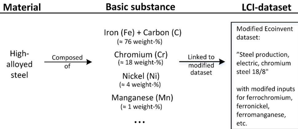
**Fig. 3.** The approach used to model the production of steel is illustrated. Basic substances composing the average blends of high alloyed steel grades, e.g., stainless steels, present in the reference option, are linked to a modified inventory dataset for high-alloyed steel production with corresponding mass shares for the final constituents, to represent the production of high alloyed steel. A similar approach is employed for the modelling of cast iron.
