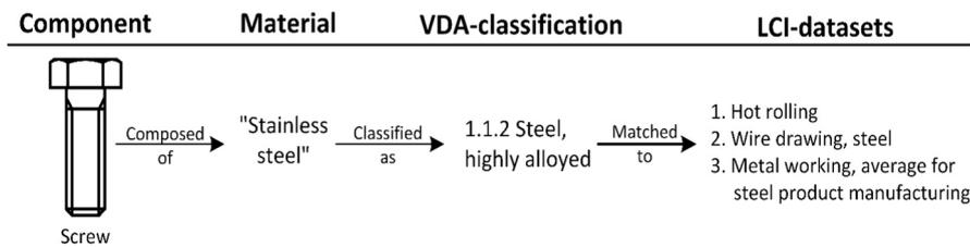
**Fig. 4.** In this example, three LCI-datasets are used to represent the manufacturing processes of a stainless steel screw: hot-rolling, followed by wire drawing and finally machining. The name of the component and the material entry, its VDA-classification as well as expert judgement are used to select suitable LCI-datasets to represent manufacturing processes in this study.
