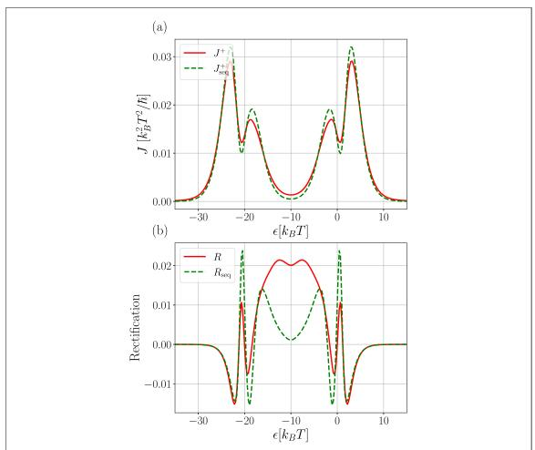
Figure 10. Closed-circuit setup. Heat currents (in units of  $k_{\rm B}^2 T^2/\hbar$ ) and rectification coefficient for the case of two non-degenerate levels as functions of the average energy of the levels  $\epsilon$ . Panel (a) shows the forward heat current and panel (b) shows the rectification R. Same color code as in figure 7. All parameters are the same used for figure 3, while  $\Delta \epsilon = 2k_{\rm B}T$  and  $E_{\rm C} = 20k_{\rm B}T$ .
