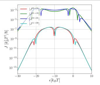
**Figure 19.** Closed-circuit setup. Heat current contributions (in units of  $k_B^2 T^2/\hbar$ ) for the case of two non-degenerate levels as functions of the average energy of the levels  $\epsilon$ . All parameters are the same used for figure 3, while  $\Delta \epsilon = 2k_B T$  and  $E_C = 20k_B T$ .
