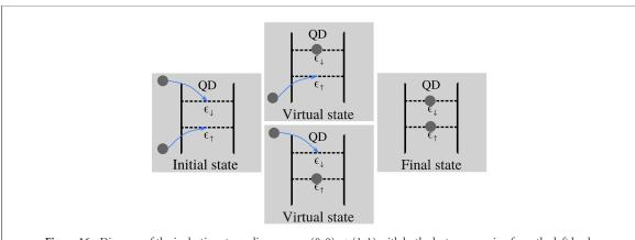
**Figure 16.** Diagram of the inelastic cotunneling process  $(0,0) \rightarrow (1,1)$  with both electrons coming from the left lead.
