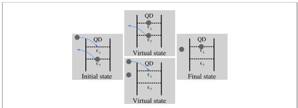
**Figure 18.** Diagram of the inelastic cotunneling process  $L \to L$  with incoming electron of spin  $\uparrow$  and QD initially in (0,1).
