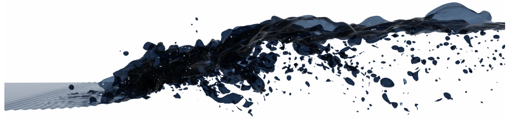
Figure 1. Classical hydraulic jump at Fr_1 = 2 ; a snapshot of the air–water interface.
