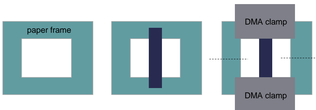
Figure 2.6 A rectangle is cut out from a sticky paper frame with the same height as the desired gauge length. After supporting the sample with a paper frame, the frame + sample are mounted in a DMA instrument followed by cutting the sides of the frame prior to measurement.
