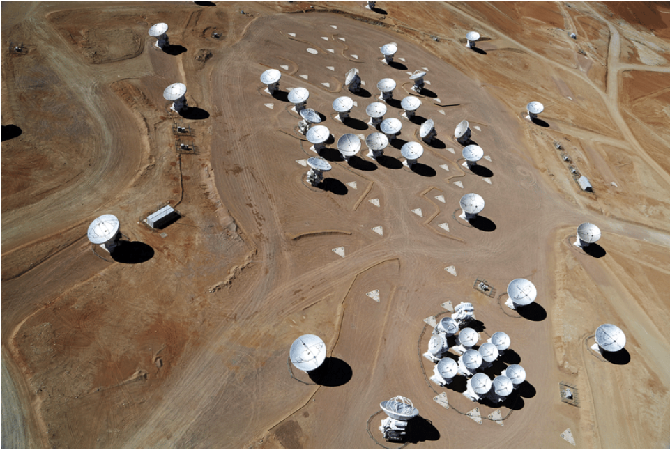
Figure 5.2: Aerial view of the ALMA telescope in the Atacama desert. Most dishes in the image are 12m main-array antennas while the small cluster in the lower right corner are the 7m dishes of the ACA. Figure from ESO.
