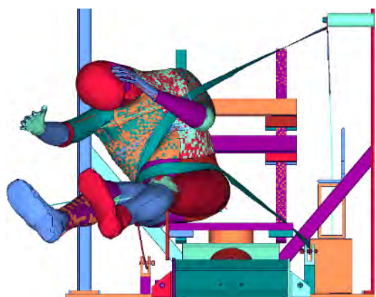
Fig. 6. Simplified far-side impact validation set-up. Snapshots at 120 ms. Configuration 1. SAFER HBM (left) and the two PMHS tests S0124, S0135 from [12].
