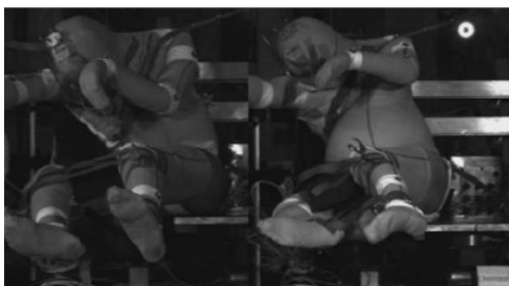
Fig. 6. Simplified far-side impact validation set-up. Snapshots at 120 ms. Configuration 1. SAFER HBM (left) and the two PMHS tests S0124, S0135 from [12].
