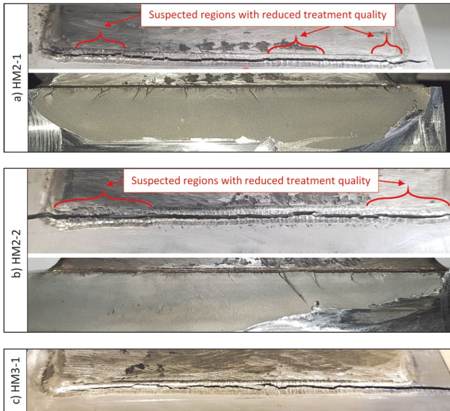
Fig. 15 Final cracks in a) HM2-1 and b) HM2-2 specimens, which failed earlier than expected ( D_{\text{real}} = 0.3 and 0.6 respectively), and c) HM3-1 specimen, which failed later than expected ( D_{\text{real}} = 1.9 )
