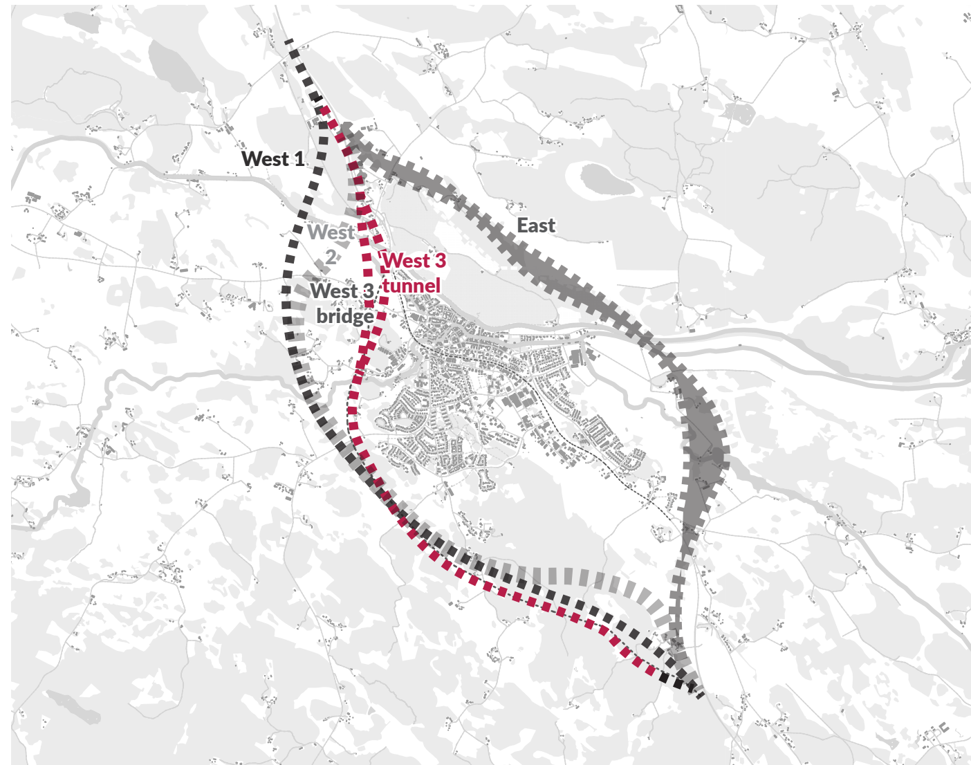
Figure 26. Case study Söderköping with the four scenarios for the planned bypass (Vägverket, vägutredning 2000-11) In red the scenario included in the before-after analysis.
