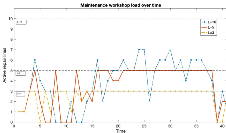
Fig. 6 Maintenance workshop load over time for (I, J_i, K, T, \underline{b}^i) = (5, 15, 10, 40, 1) and L \in \{10, 5, 3\} . Points on the Pareto front for objectives (10) and (8): availability = 5; maintenance cost \in \{5542, 5546, 5631\} ; no constraints on the stock levels at the end of the planning horizon
