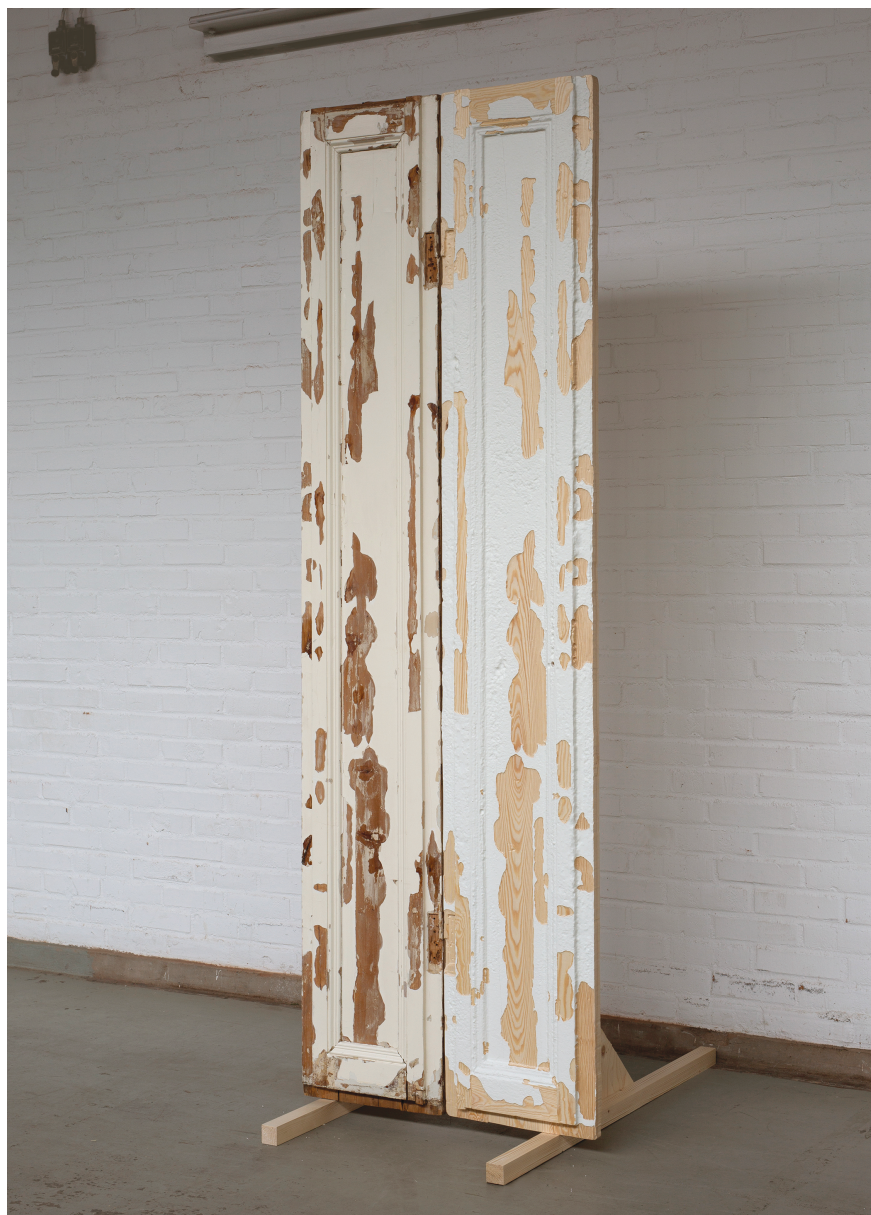
Figure 3.6. Daniel Norell, Einar Rodhe, and Karin Hedlund, Completions , double door panel, 2020. 3d-scanning and CNC-routing are used to create a replica (right) of an existing double door panel (left), including wear and tear.
