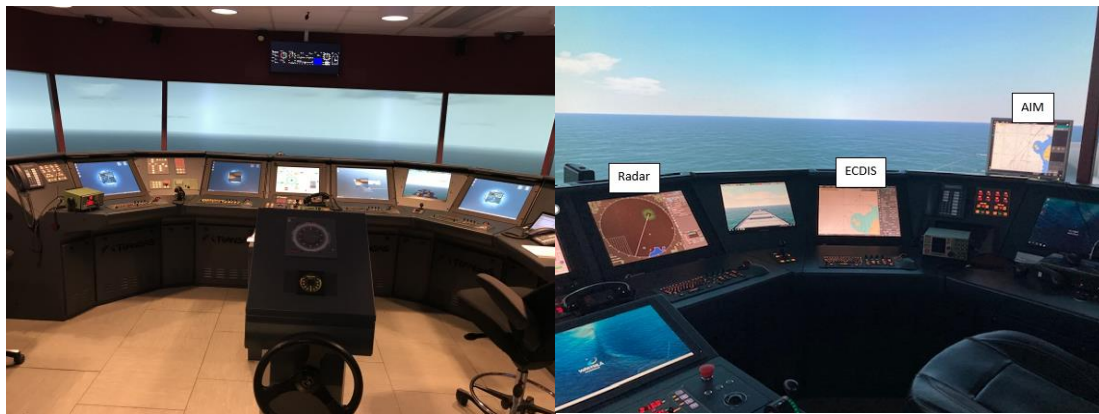
Figure 7 (Left) High-fidelity ship's bridge simulator at Chalmers University of Technology (Right) The test-set up for Paper III with the additional decision support screen.
