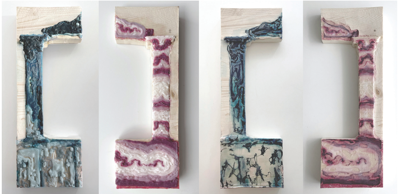
11 Left: Initial aesthetic outcomes of architectural element retrofitting with microfibrillated cellulose hydrogel (fully wet prototypes, 30 minutes after 3D printing). Right: Final aesthetic outcomes of architectural element retrofitting with microfibrillated cellulose hydrogels (fully dried prototypes, 36 hours after 3D printing).
