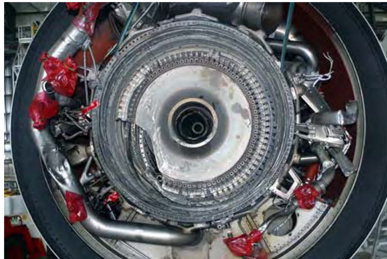
Figure 1.1: Rear face of the broken stage-1 HPT disk from a Boeing 767-219ER (General Electric CF6-80A high-bypass turbofan engine). The fracture originated on the left side of the disk, the initial part of the crack broke intergranularly. [1]
