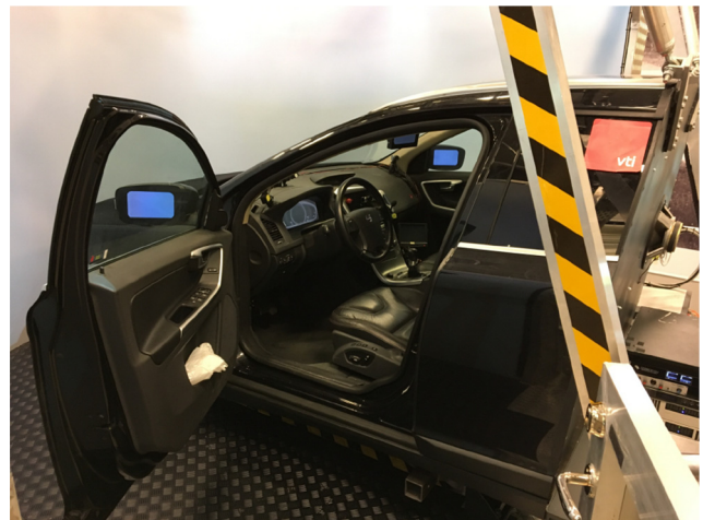
Figure 2 Passenger car cabin of the “SimIV” driving simulator
