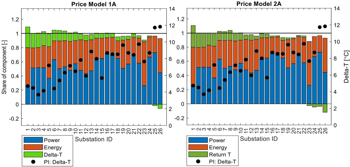
**Figure 24:** Share of price model components for new price model 1A with a delta-T component, and price model 2A with a return temperature component, replacing the flow component of the existing price model (Jangsten, Lindholm, and Dalenbäck 2022b).
