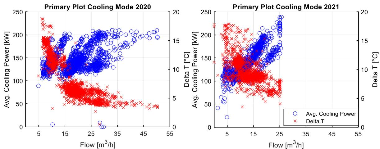
**Figure 19:** Evaluation of flow limitation control strategy as tested in one building. Left: reference period without the flow limitation control strategy. Right: test period with the control strategy (Jangsten, Lindholm, and Dalenbäck 2022c).
