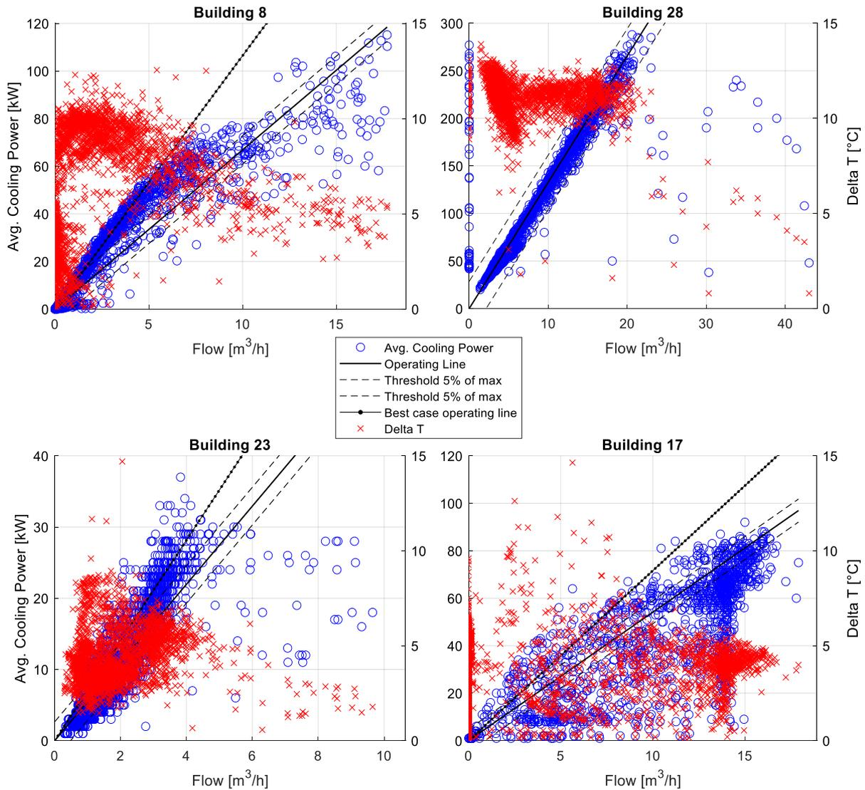
**Figure 9:** Example of primary plot with reference model for four different substations. Building 8 is based on data from 2021 and buildings 28, 23 and 17 are based on data from 2018. The figure is adopted from Jangsten (2020) and Jangsten, Lindholm, and Dalenbäck (2022a).
