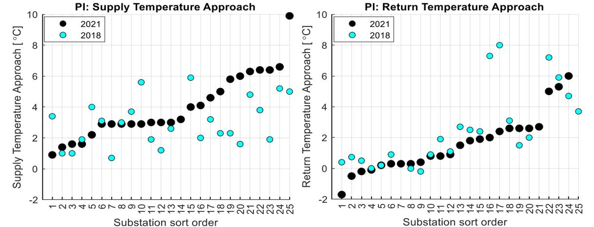
**Figure 13:** Performance indicators supply temperature approach (left) and return temperature approach (right) for 25 substations from the cooling seasons of 2018 and 2021 (Jangsten, Lindholm, and Dalenbäck 2022a).
