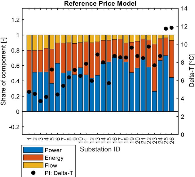
**Figure 23:** Reference price model: shares of components for 26 analyzed substations. Also, shown is the performance indicator (PI) delta-T for peak cooling loads (Jangsten, Lindholm, and Dalenbäck 2022b).
