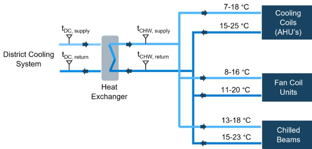
**Figure 17:** Typical configuration of the chilled water systems of the buildings connected to the district cooling system, with subsystems and associated supply and return temperatures (Jangsten et al. 2020).
