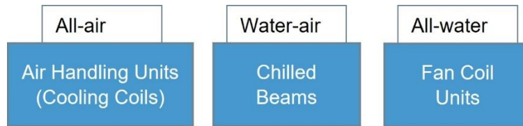
Figure 4: Classification and type of building HVAC system in the buildings part of this thesis.
