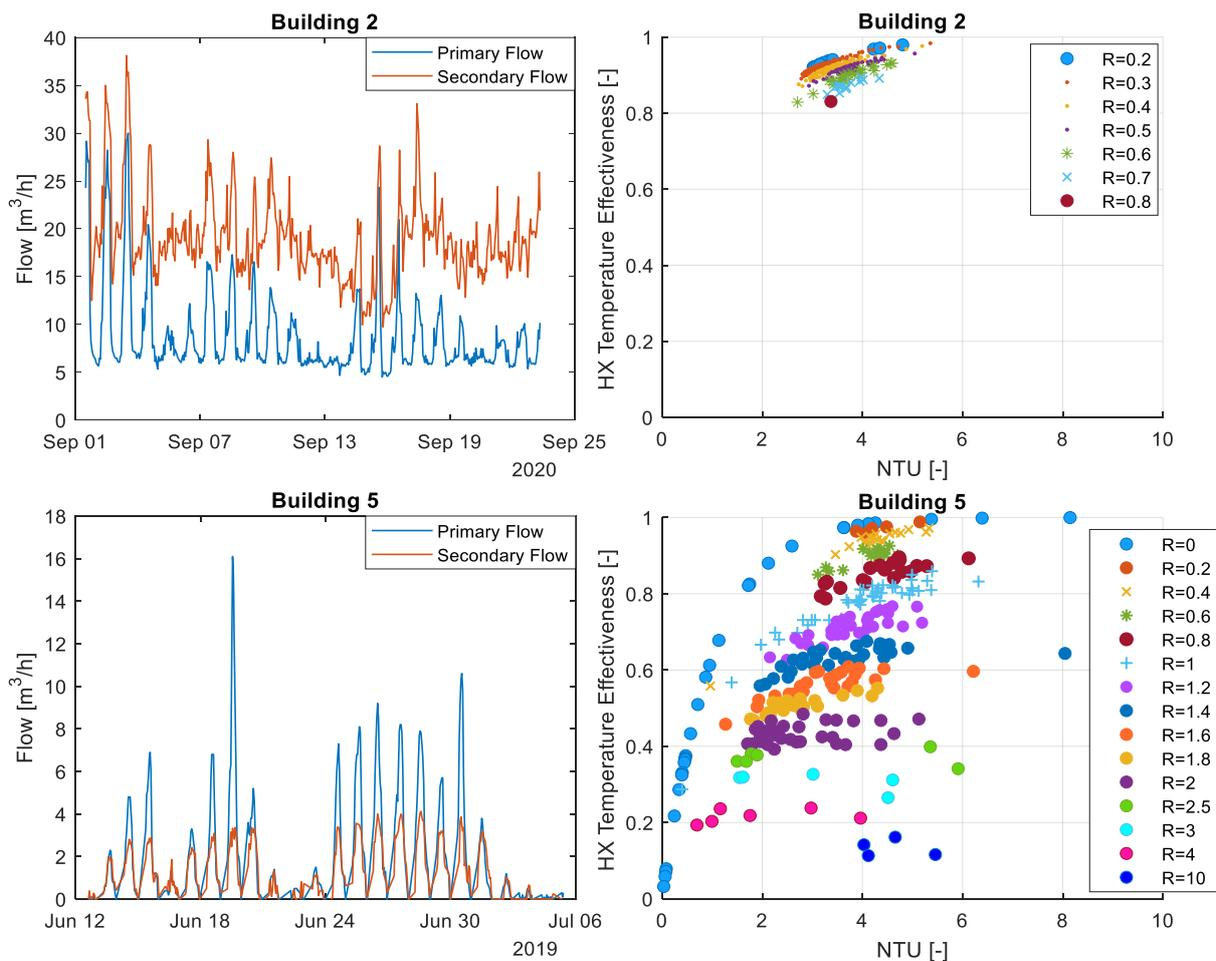
**Figure 15:** Left: primary flow rates and secondary flow rates from field measurements for buildings 2 and 5. Right: Heat exchanger temperature effectiveness as a function of NTU and flow rate ratio R for buildings 2 and 5 (Jangsten, Lindholm, and Dalenbäck 2022c).
