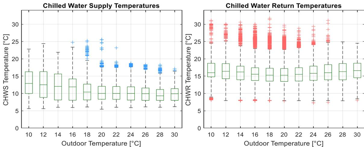
**Figure 16:** Boxplot of the actual chilled water supply and return temperatures on the secondary side of the heat exchanger in the substation for 11 outdoor temperature categories. Each data point is an hourly measurement recorded during April to September of 2018. Left: chilled water supply (CHWS) temperatures. Right: chilled water return (CHWR) temperatures (Jangsten et al. 2020).
