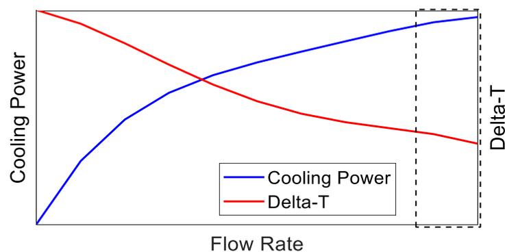
**Figure 7:** Theoretical “primary plot” which is a correlation plot of cooling power, flow rate and delta-T of the primary side of the substation, with saturation zone indicated by dashed lines (Jangsten 2020).
