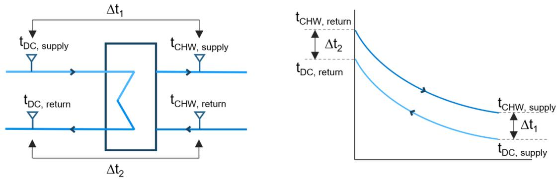
**Figure 3:** Schematic of temperatures and temperature approaches in a district cooling substation along with temperature diagram for counterflow heat exchanger for district cooling substation applications.
