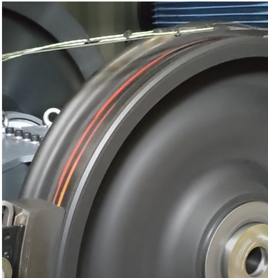
Figure 2.2: Image showing hot bands forming on the wheel treads, indicating that heat flux is not evenly distributed
