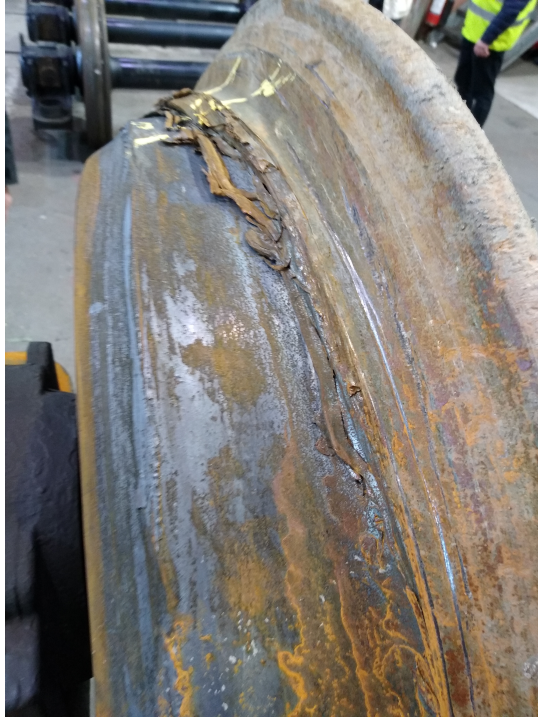
Figure 1.1: Wheel damage due to an extreme tread braking event where the running surface has been gradually worn away and material has been rolled out axially.
