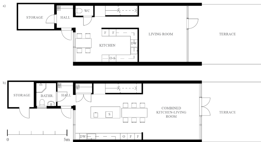
Figure 1. The floorplan of the terraced house of case I-3 before (a) and after (b) the alterations (DW: dishwasher, F: fridge or freezer, O: oven, S: stove).
