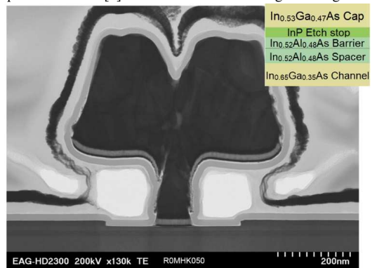
Fig. 1. STEM image of the 100 nm-length gate of the InP HEMT with d_{sp} = 3 \text{ nm} . The inset: epitaxial stack of the InP HEMT.
