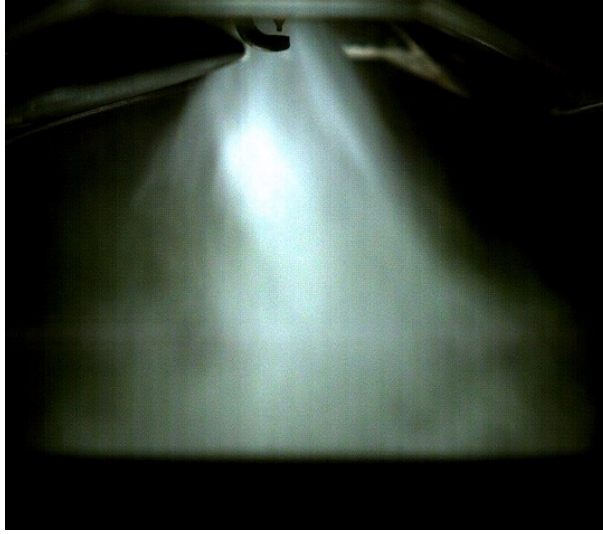
Figure 2.3: Image of a fuel spray injected into the cylinder of a GDI engine (SOI: -320 bTDC)
