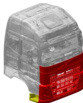
FIGURE 6 LOWER FRONT AREA (HIGHLIGHTED IN RED) OF A TRUCK CAB
