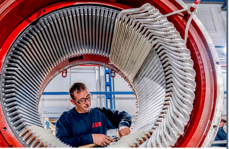
High voltage motors are often used until failure, with one of the most common faults occurring in the stator copper windings.
