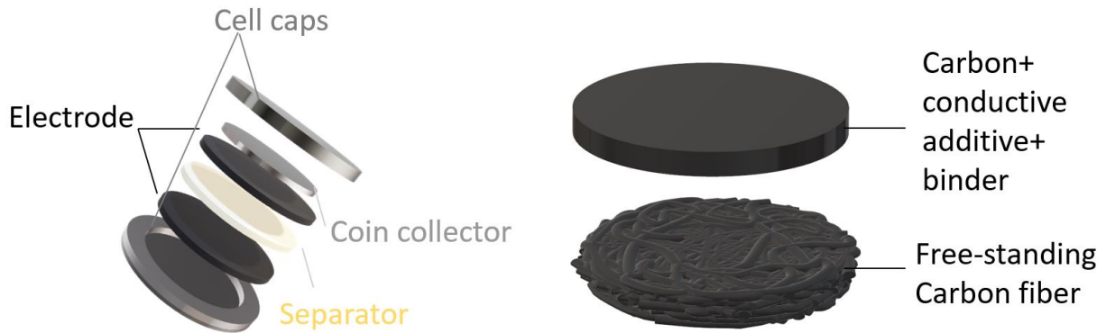
Figure 12. Schematic representation of a coin cell and its different components with some of their different electrode forms.
