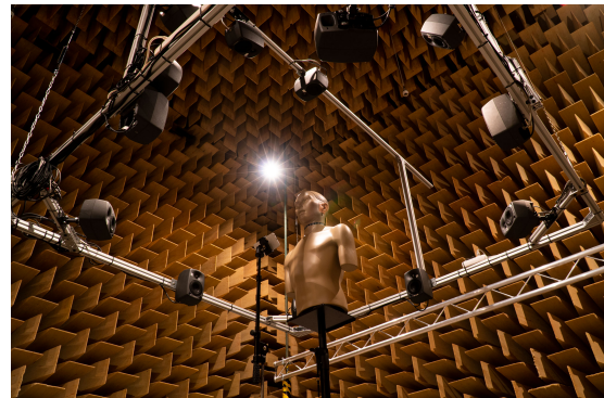
Fig. 2: Loudspeaker setup in anechoic chamber with artificial head at participant position and smart-phone mounted in front of participant
