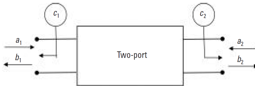
Figure 17: Illustration of the noise waves associated with a linear two-ports device – from [97]
