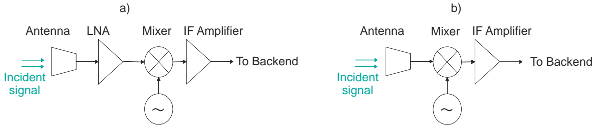
Figure 1: Illustration of typical radio-astronomy receivers. a) configuration used for frequencies up to around 100 GHz b) configuration used for above 100 GHz.
