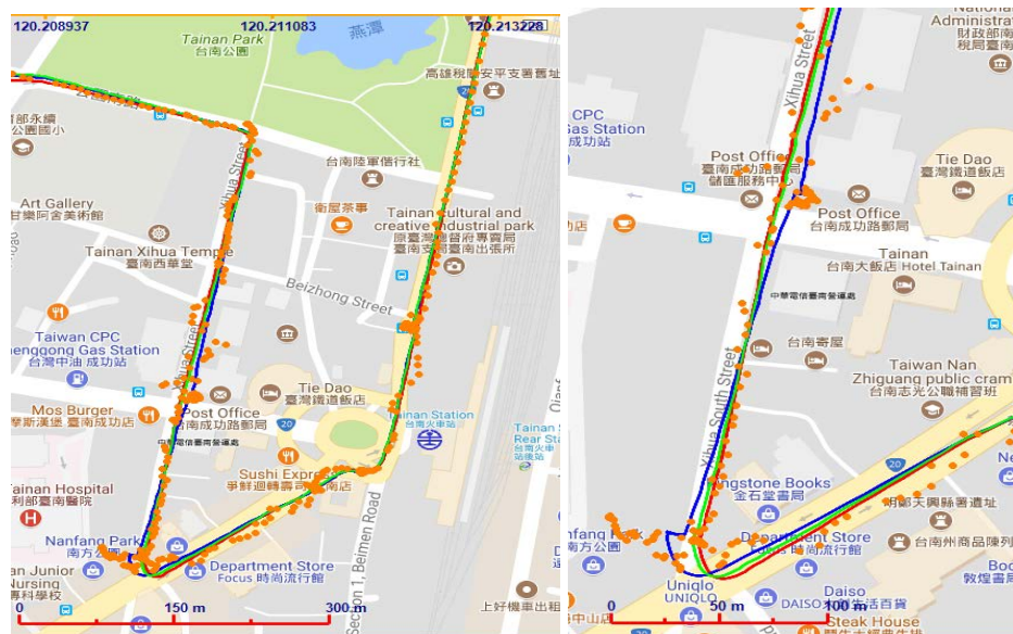
Fig. 3: Trajectories of three different results; SPAN-LCI (red line), C-MIGITS with ublox GPS (blue line), real-time SLAM-aided solution (green line), GNSS points (orange); SLAM-aided part (right) and enlarged SLAM-aided area.
