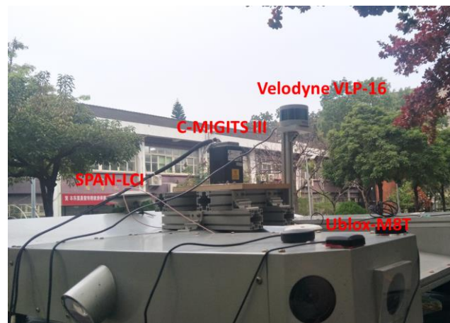
Fig. 2: Land vehicle positioning payload.
