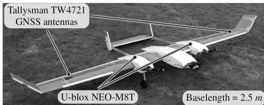
Fig. 1: UAV with the mounted GNSS sensors.
