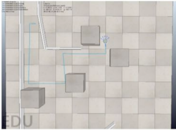
Fig. 17. Simulating obstacle avoidance behaviour robot with Ultrasonic sensor and K.F algorithm in V-rep software
