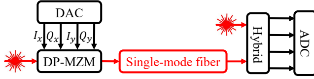
Figure 5.3: Single carrier transmission over a single-mode fiber. In this case, the multidimensional constellations are realized over two polarizations, IQ components, and multiple time slots in a single carrier.
