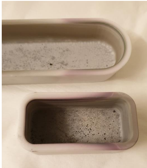
Figure 6.15. Alumina crucibles used as sample holders after carbothermic reduction and nitridation of the Cr-doped microspheres. Pink coloration was observed on the edge, suggesting a possible reaction with Cr.
