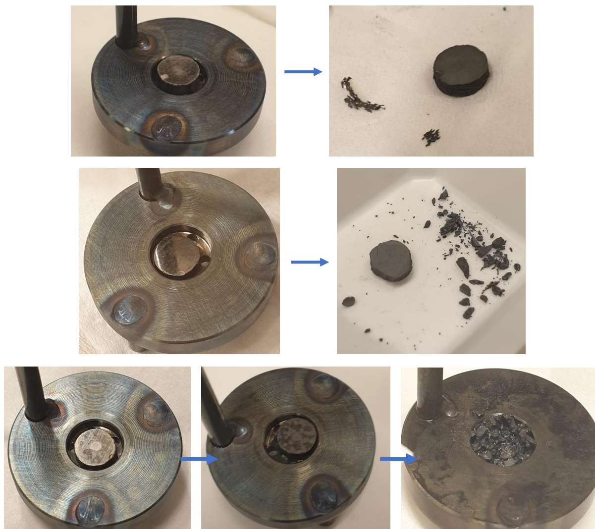
Figure 6.28. Photographs of (U80Cr20)N-3 (top), U80Cr20N-13 (middle), and U80Cr20N-23 (bottom) Cr-doped UN pellets from Batch A and B before and after exposure to water at 300\text{ }^{\circ}\text{C} . The U80Cr20N-23 pellet was exposed for 3 extra hours, after which crumbling occurred.
