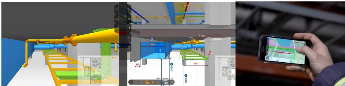
FIG. 2: Site-workers can use mobile devices to navigate in either 2D or 3D to their current work area and create unlimited sections and measurements in the same view (Image from case projects: Lumi and Celsius).
