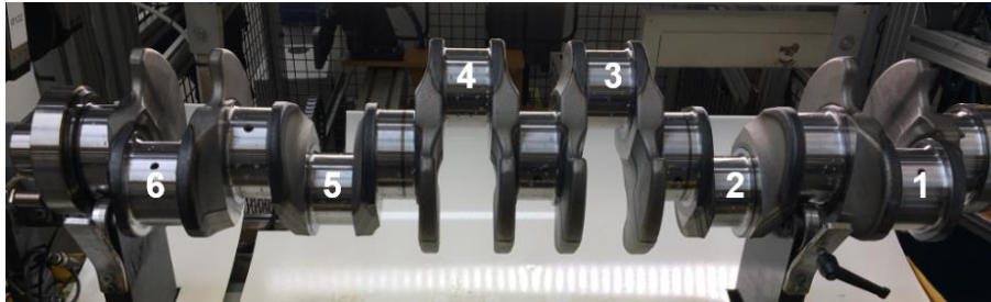
Fig. 40. Crankshaft with labelled crankpins were the focus parts in the grinding process.
