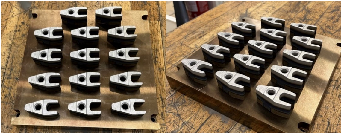
Figure 2: Example of injector yokes (Volvo AB) that were made from AISI 4140 low-alloy steel and produced by PBF-LB.
