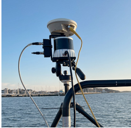
Fig. 3. The sensor platform setup containing an Ouster-OS2-128 lidar and GNSS antenna.
