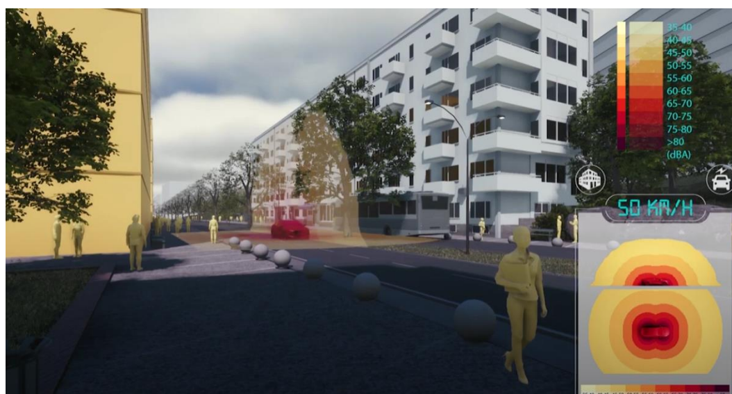
Figure 2: Illustration of the visualisation/auralisation tool in use with dynamic real-time noise levels illustrated with transparent coloured surfaces.
