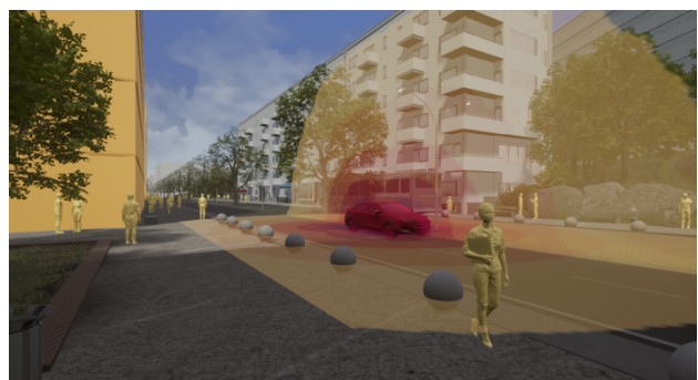
Figure 3. Visualization of noise in the project with a colour scale ranging from lighter yellow to darker red, where red symbolizes the strongest noise area and yellow the weakest.
