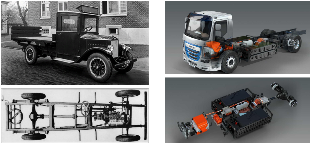
Figure 1.1: Illustration of a 4x2 vehicle configuration, with chassis mounted prime mover and rear axle drive; (left): Historical diesel engine layout on Volvo ÖV4 TV pickup vehicle from 1927 [21]. (right): DAF LF Battery Electric Innovation Truck exhibited at IAA 2018 [7].
