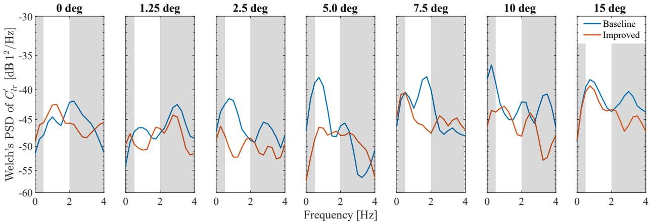
**Figure 5.5:** Welch's PSD (power spectral density) frequency response of the rear lift fluctuations ( $C'_{lr} = C_{lr} - \overline{C_{lr}}$ ) for the two spoilers at 0, 1.25, 2.5, 5, 7.5, 10 and 15 deg yawed flow angle. Using 2s window size and 90% overlap.
