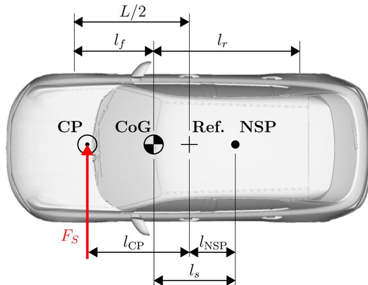
**Figure 2.3:** Top view of a vehicle visualising the typical longitudinal positions of the aerodynamic centre of pressure (CP), the centre of gravity (CoG), a geometric reference point between the axles (Ref.) and the neutral steering point (NSP).
