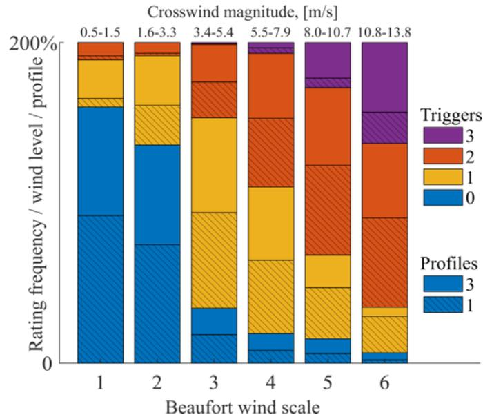
**Figure 4.5:** The occurrence frequency of each trigger rating for crosswind gusts ranging from 1 to 6 on the Beaufort scale. Gust profiles 1 and 3 separately accumulate to 100% for every crosswind level.
