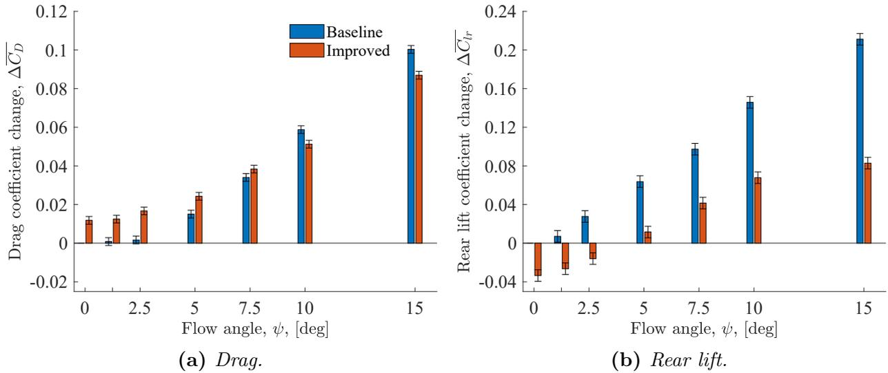
**Figure 5.2:** The influence of roof spoiler design and yawed flow angle on the aerodynamic coefficients, with the baseline spoiler at zero flow angle as reference. Numerical uncertainties were estimated based on averaging time, and the mesh and time step study in Paper C.
