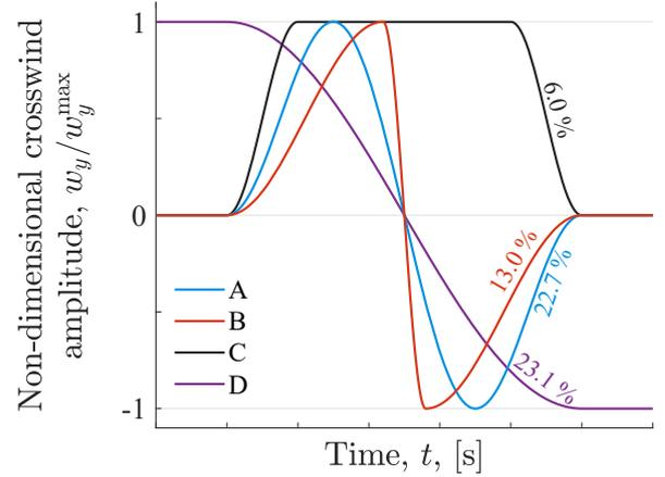
**Figure 3.6:** The four gust classes (A-D) classified in the experimental study and their frequency of occurrence (35.2% undefined).
