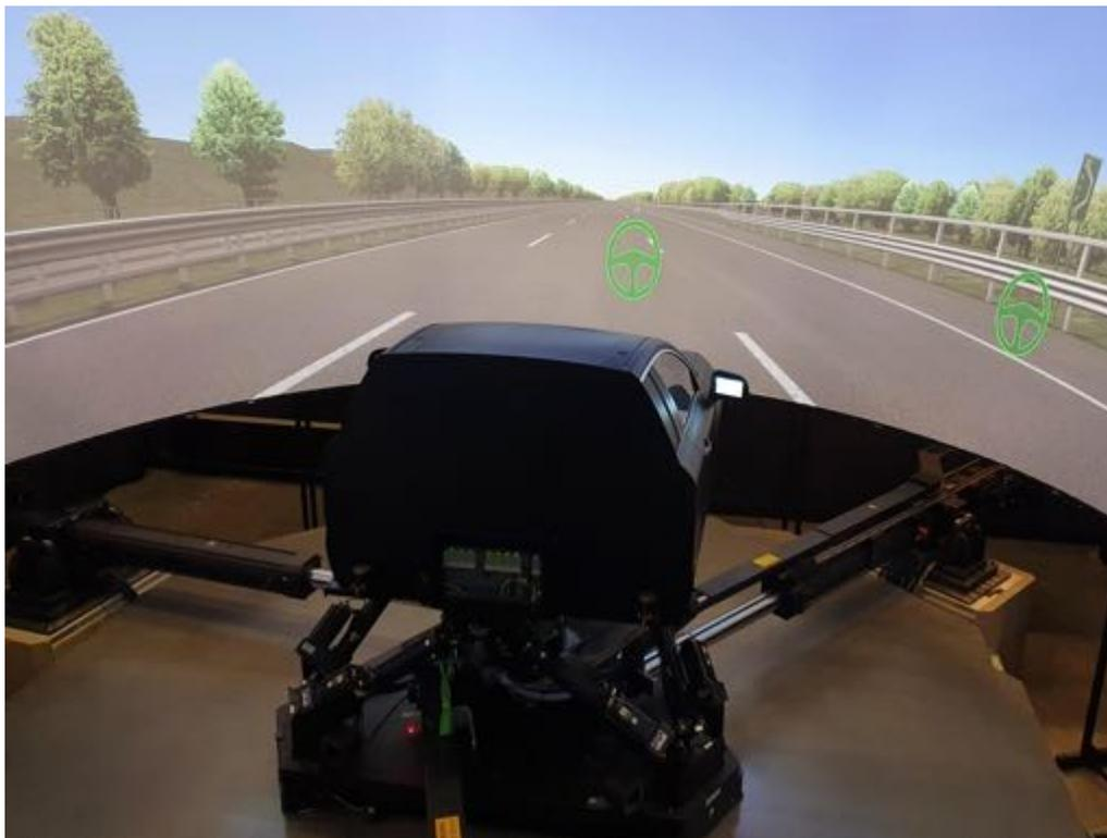
**Figure 3.14:** *The VI-grade DiM250 driving simulator at CEVT.*
