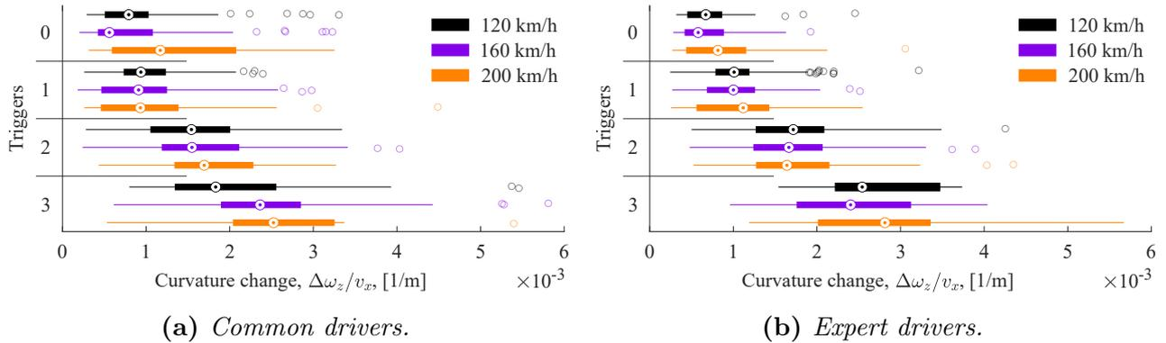
**Figure 4.8:** Boxplots of the path curvature change per trigger level, for (a) common and (b) expert drivers at 120, 160 and 200 km/h. The thick lines represent the interquartile range between the lower and upper quartiles with the circled dot as the median. Outliers are shown as circles.
