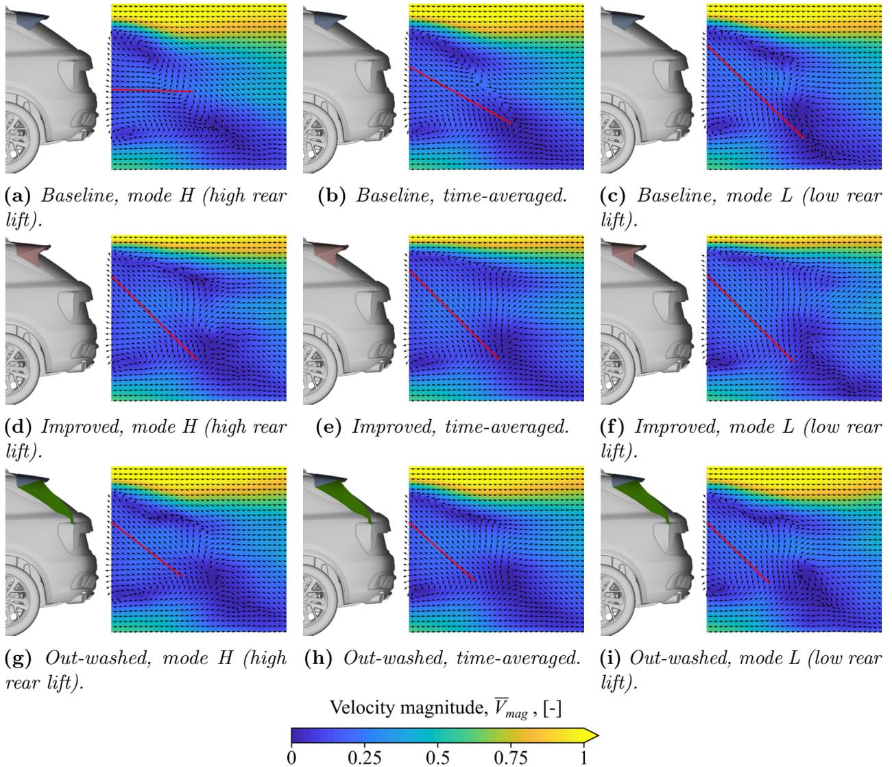
**Figure 5.16:** Conditionally averaged wake velocity fields for the high (H) and low (L) rear lift modes, at 5 deg yawed flow. Time-averaged velocity fields are included for comparison in the  $y$ -normal centreline planes. The red lines are manually positioned in the overall flow direction towards the base to mark the wake balance.
