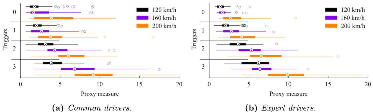
**Figure 4.7:** Boxplots of the proxy measure (Equation 4.1) per trigger level, for (a) common and (b) expert drivers at 120, 160 and 200 km/h. The thick lines represent the interquartile range between the lower and upper quartiles with the circled dot as the median. Outliers are shown as circles.
