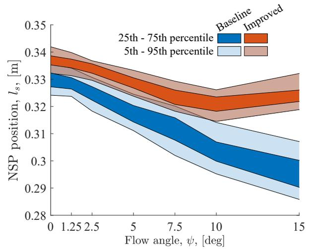
**Figure 5.11:** The neutral steering point (NSP) variations, relative CoG, for the two spoilers at  $\psi = 0, 1.25, 2.5, 5, 7.5, 10$  and  $15$  deg.
