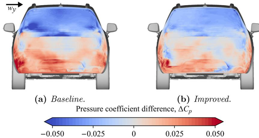
**Figure 5.8:** Conditionally averaged base pressure differences between the high ( $H$ ) and low ( $L$ ) rear lift modes, for the two spoilers at 5 deg yawed flow.
