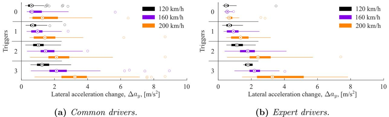
**Figure 4.6:** Boxplots of the lateral acceleration response per trigger level, for (a) common and (b) expert drivers at 120, 160 and 200 km/h. The thick lines represent the interquartile range between the lower and upper quartiles with the circled dot as the median. Outliers are shown as circles.
