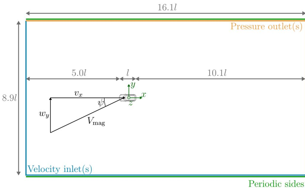
**Figure 3.4:** Top view of the computational domains with inlet, outlet and periodic boundaries marked in blue, orange and green, respectively. The relations between the flow angle,  $\psi$ , flow velocity,  $V_{mag}$ , vehicle velocity,  $v_x$ , and lateral wind component,  $w_y$ , are shown.
