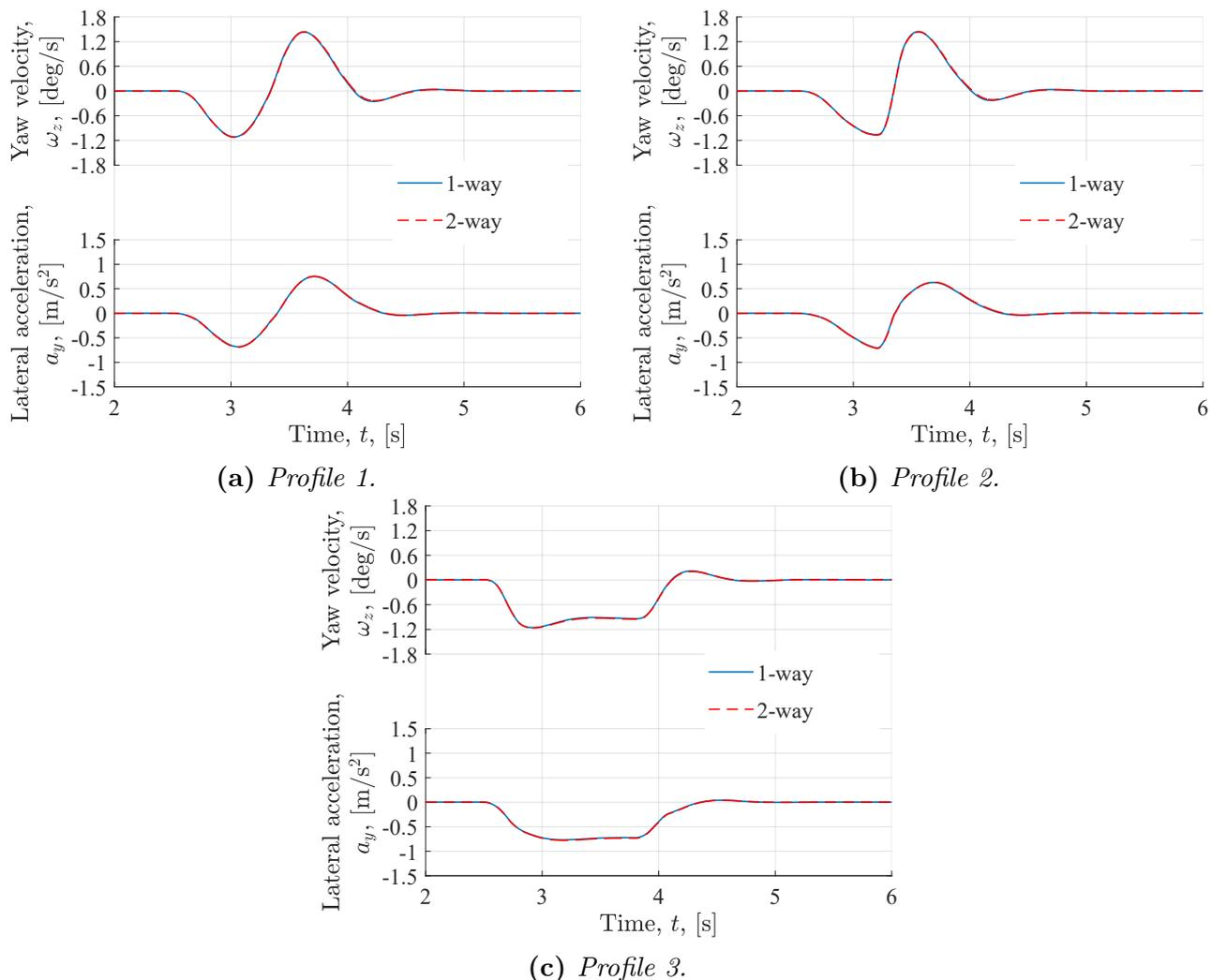
**Figure 3.13:** The vehicle motion response in terms of yaw velocity,  $\omega_z$ , and lateral acceleration,  $a_y$ , for the three gust profiles, comparing 1-way and 2-way coupled solutions for the SUV.
