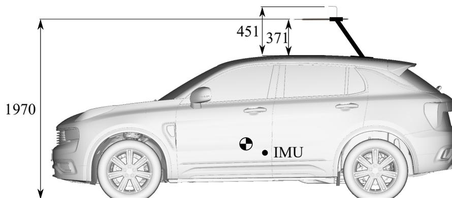
**Figure 3.15:** *Schematics of the placement of the seven-hole probe and the Prandtl tube in mm and the position of the inertial measurement unit (IMU).*
