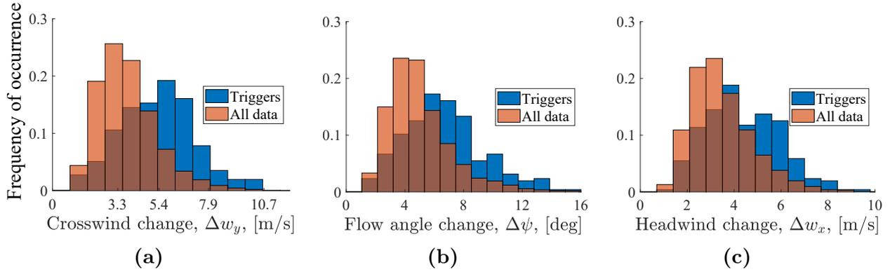
**Figure 4.1:** The frequency of occurrence distributions for three wind quantities, comparing the data at the trigger events to the complete data set.
