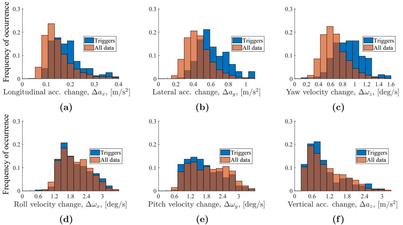
**Figure 4.2:** The probability of occurrence distributions for six vehicle motion quantities, comparing the data at the trigger events to the complete data set.
