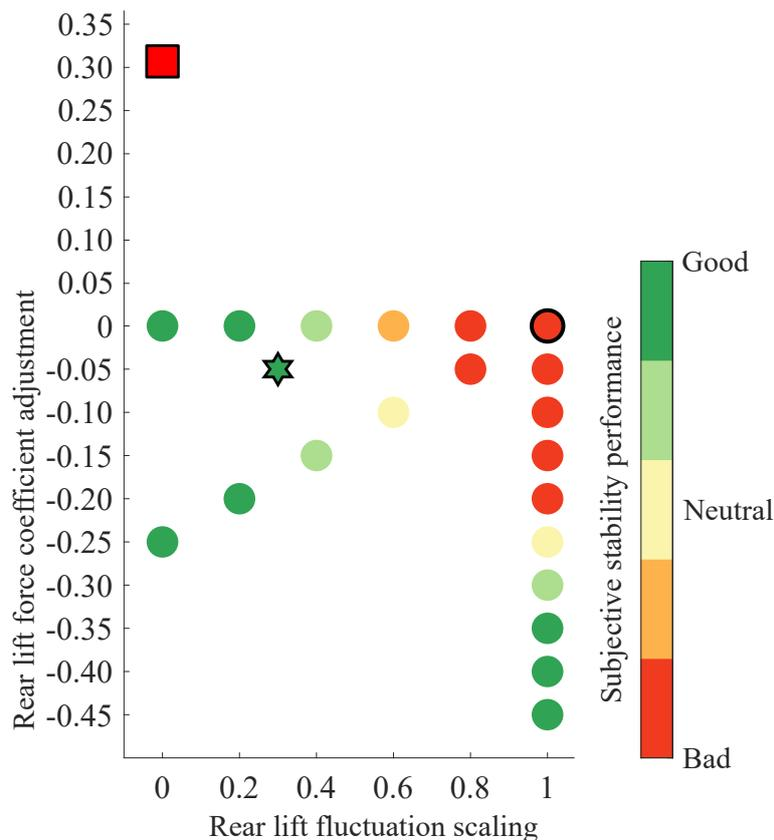
**Figure 5.19:** *The effects of time-averaged rear lift and rear lift fluctuation amplitude on the subjective high speed stability performance. The circle represents the baseline spoiler (configuration 1.1.), the star is the improved spoiler (configuration 2.2) and the square estimates the required rear lift coefficient making the linear system of the bicycle model unstable.*
