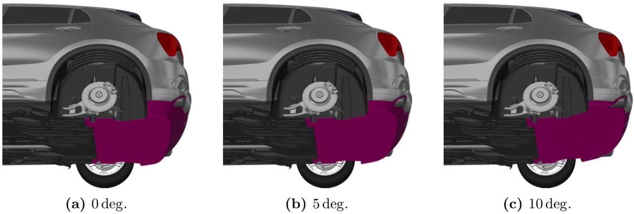
**Figure 5.12:** Rendered images of the three diffusers (purple) on the test vehicle equipped with the baseline spoiler.
