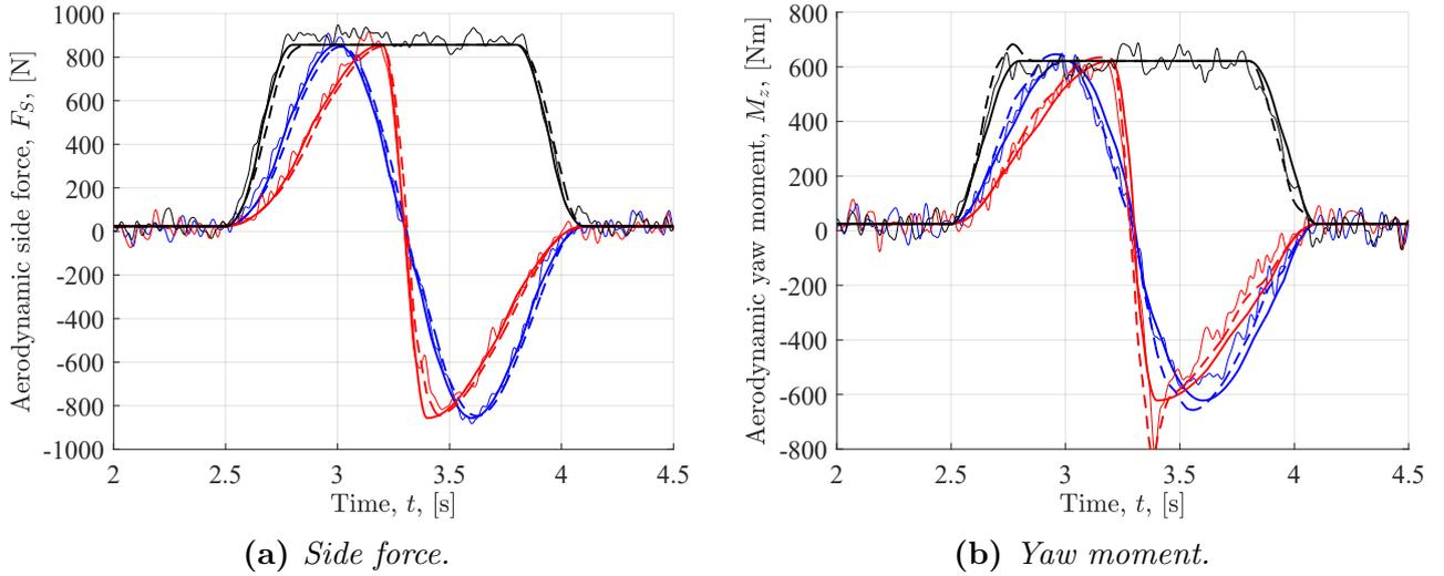
**Figure 3.7:** The aerodynamic response for gust profile 1 (*blue*), profile 2 (*red*) and profile 3 (*black*), comparing tCFD (thin lines —) to QS (thick lines —) and QSD (thick dashed lines ---) approaches.
