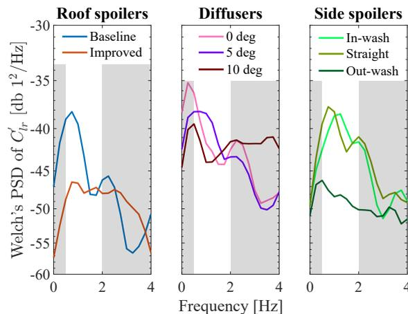
**Figure 5.14:** Welch's PSD (power spectral density) frequency response of the rear lift fluctuations ( $C'_{lr} = C_{lr} - \overline{C_{lr}}$ ) for the two roof spoilers, the three diffusers and the three side spoiler designs, at 5 deg yawed flow. Using 2 s window size and 90 % overlap.
