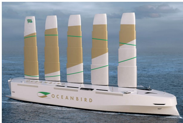
Figure 1.1: Concept design of the car carrier Oceanbird (2021).
