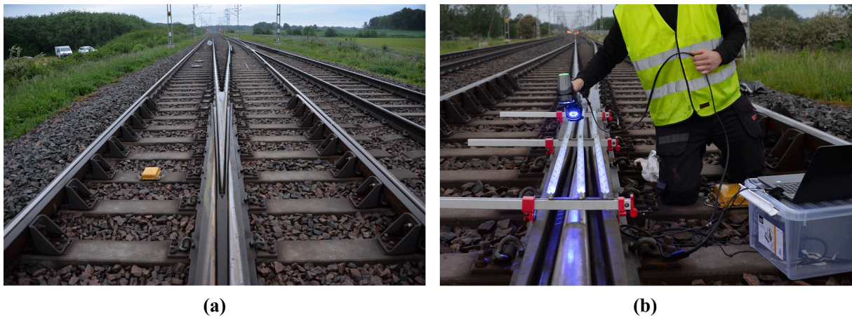
Fig. 2. (a) Accelerometer from Konux GmbH (yellow box) installed on the sleeper adjacent to the crossing transition. (b) 3D geometry scan of a crossing transition. (For interpretation of the references to colour in this figure legend, the reader is referred to the web version of this article.)
